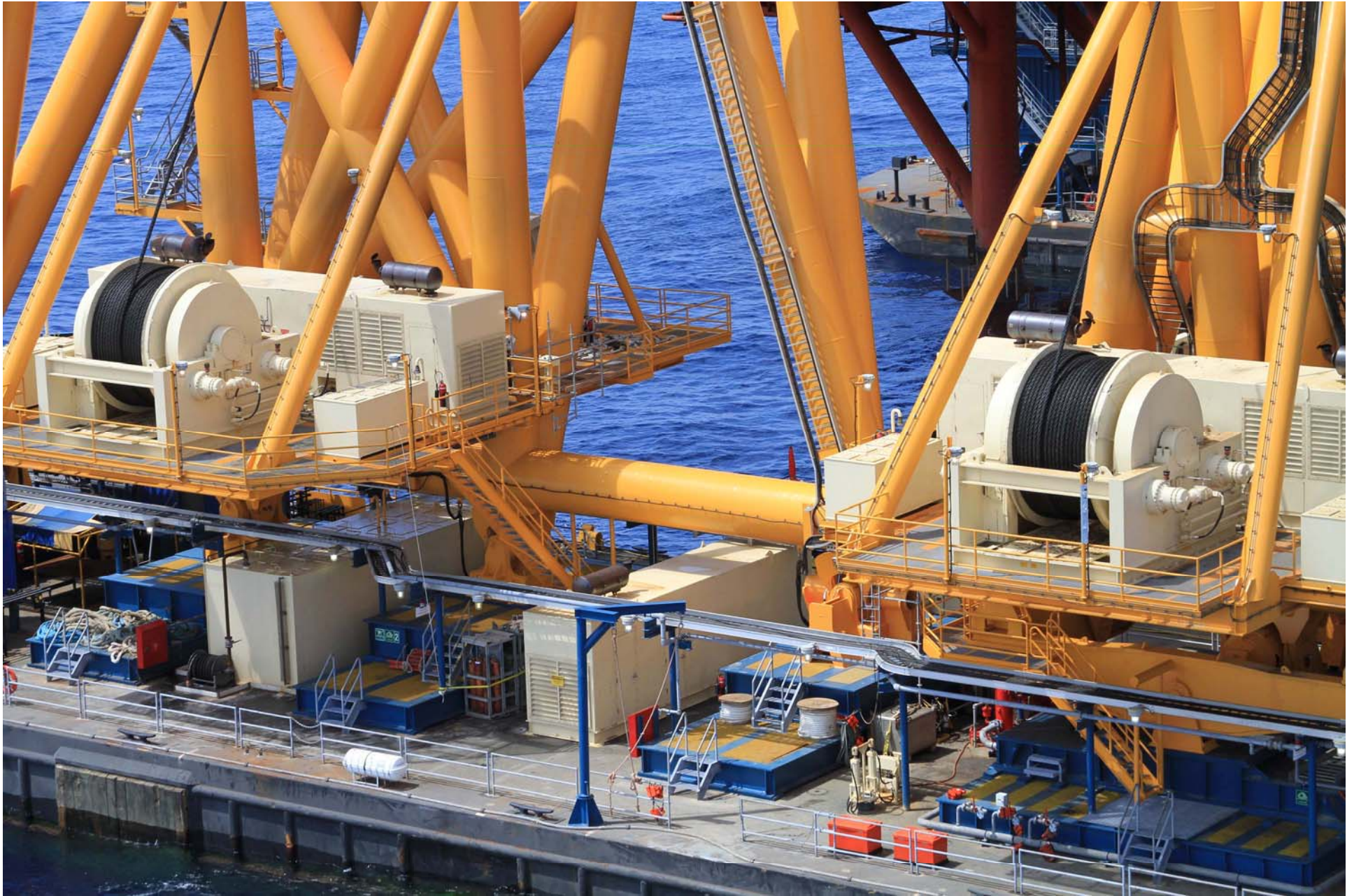
The system's four 300-ton main hoist winches, each carrying 7500 feet of 3 1/2 " wire rope, are idled up and ready to go. The VB - 10000 has a lift capacity of 7,500 tons.
