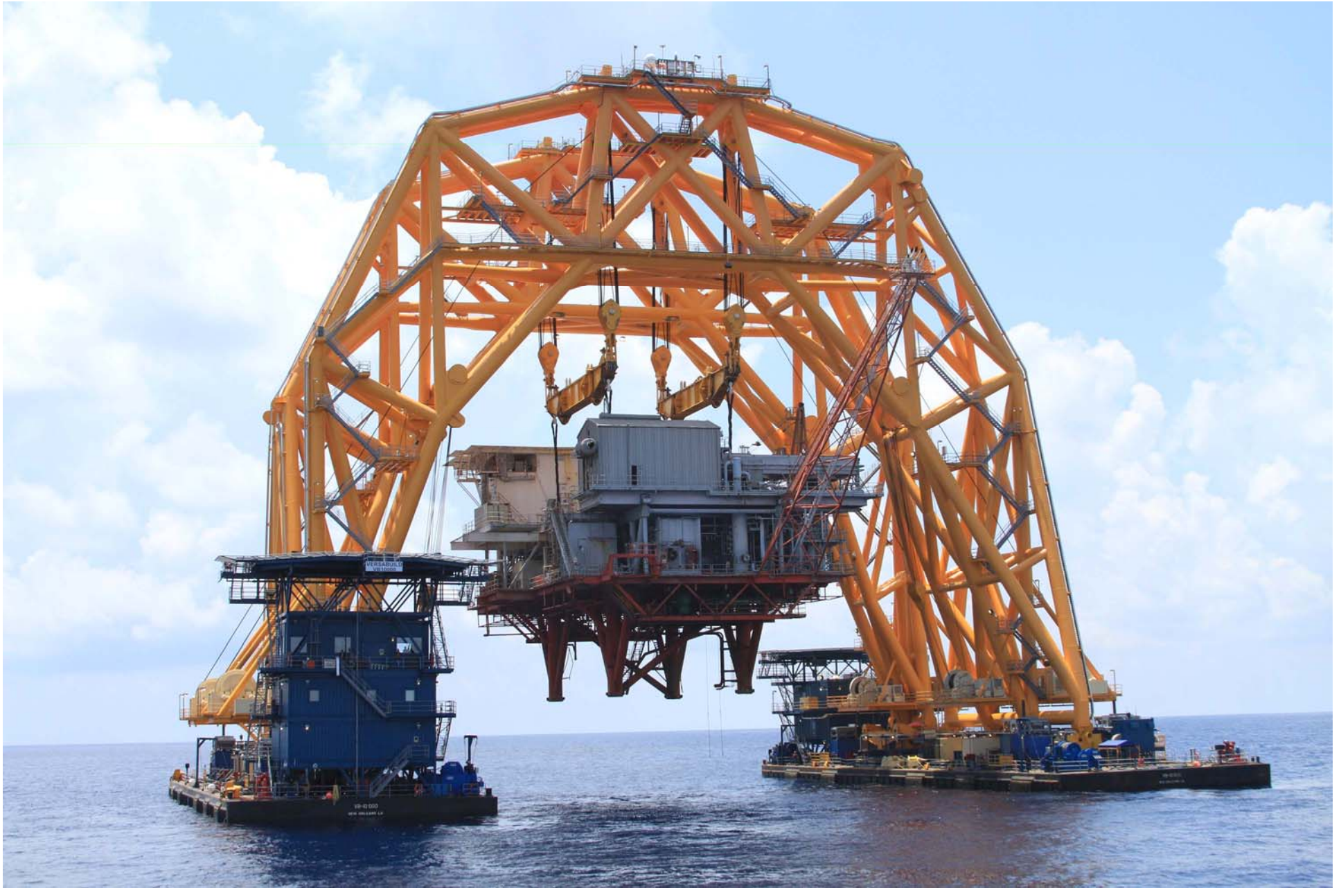
The VB – 10000's hook-height insures plenty of clearance for the barge.
